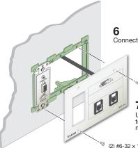
Connect the remaining cables to the AAPs.
